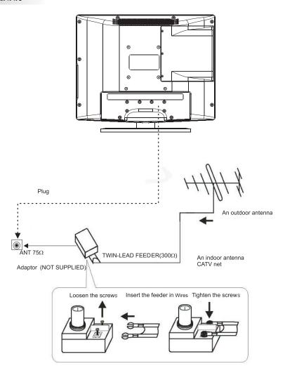
Note:  $Aerial\ connections: IEC (female). \\ Input\ impendance: 75\Omega\ unbalanced.$
